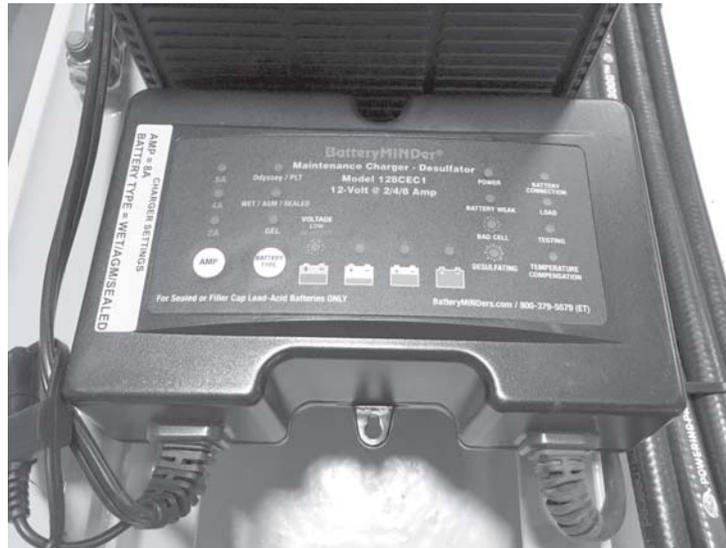
**H150E-7200-3:** This charger is fully automatic. It can be plugged in anytime the *Heliporter®* is not in use and will maintain the batteries as needed.
